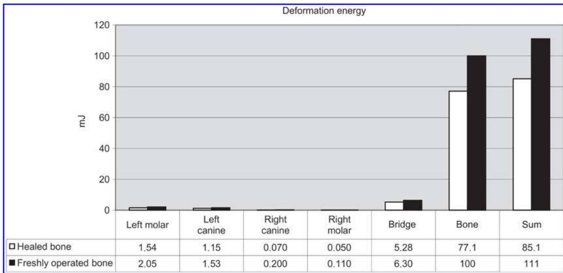
Figure 5 Absolute deformation energy stratified for healing state and components.
