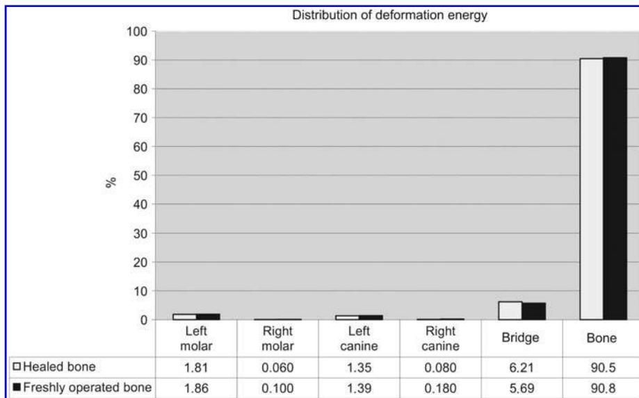
Figure 6 Relative deformation energy distribution stratified for healing state and components.
