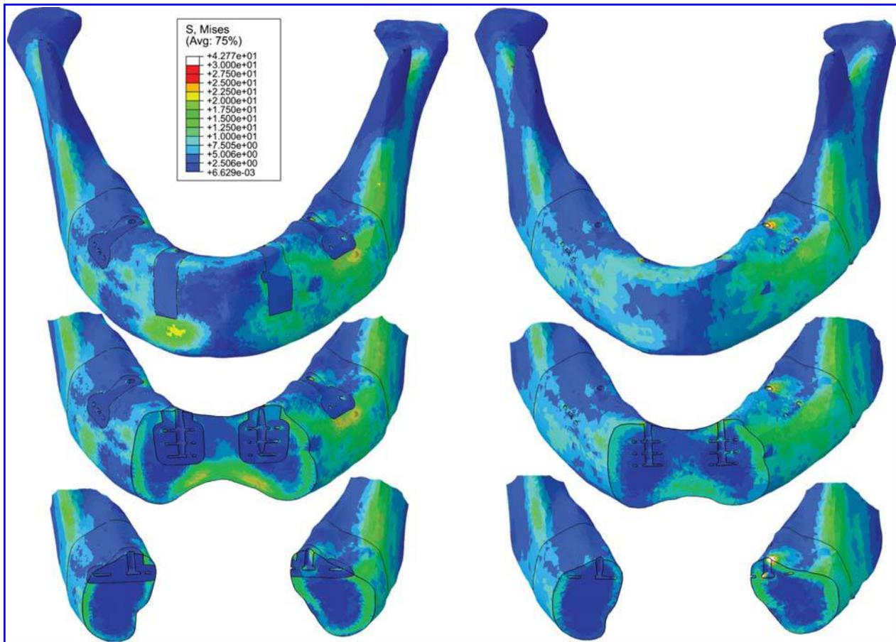
**Figure 3** von Mises stress contours. Compilation of whole mandible and vertical cross-sections through the mandible in the area of the implants. Left, fresh operated; right, healed bone.
