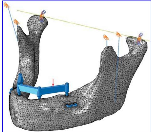
**Figure 2** Model of mandible with implants, bridge and with marked muscles, boundary conditions and loading force.
