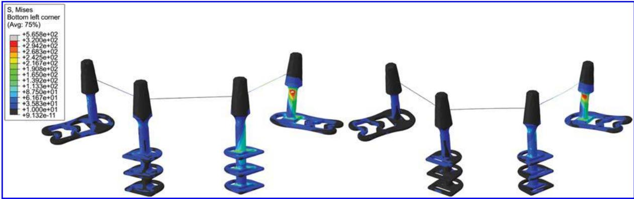
Figure 4 von Mises stress contours in all implants. Left, fresh operated; right, healed bone.
