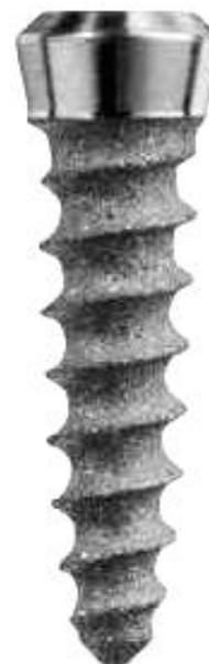
Fig 1 : The STO®-Implant provides full compatibility to the 4.8mm ITI-standard. In addition a compression screw bone thread allows aggressive tightening of the implant even in soft bone. The Osmoactive® surface helps to prevent early bacterial colonialization and the same time promotes adhesion of the blood cloth.
